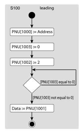
The following diagram explains the parameter reading procedure.
