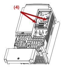
■ Mount PROFInet communication Module and fasten the removed screw(6) and the included screw(7).
