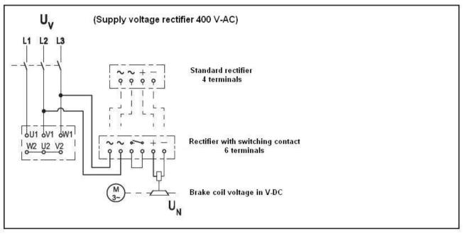
Supply: Phase-Phase Half-wave rectifier
