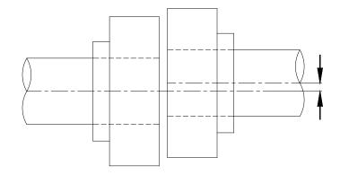
**7.3.3**- When installing the coupling, please observe the maximum permissible angular displacement.
